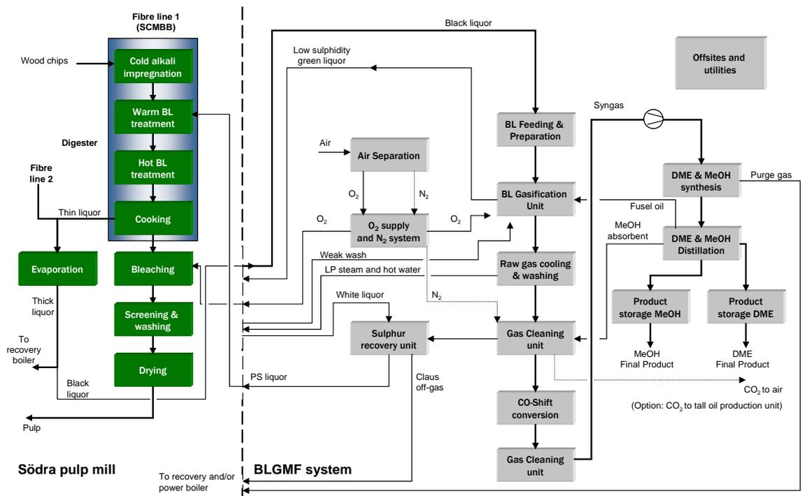
Figure 4 The BLGMF plant and its connections to the SCM pulp mill
