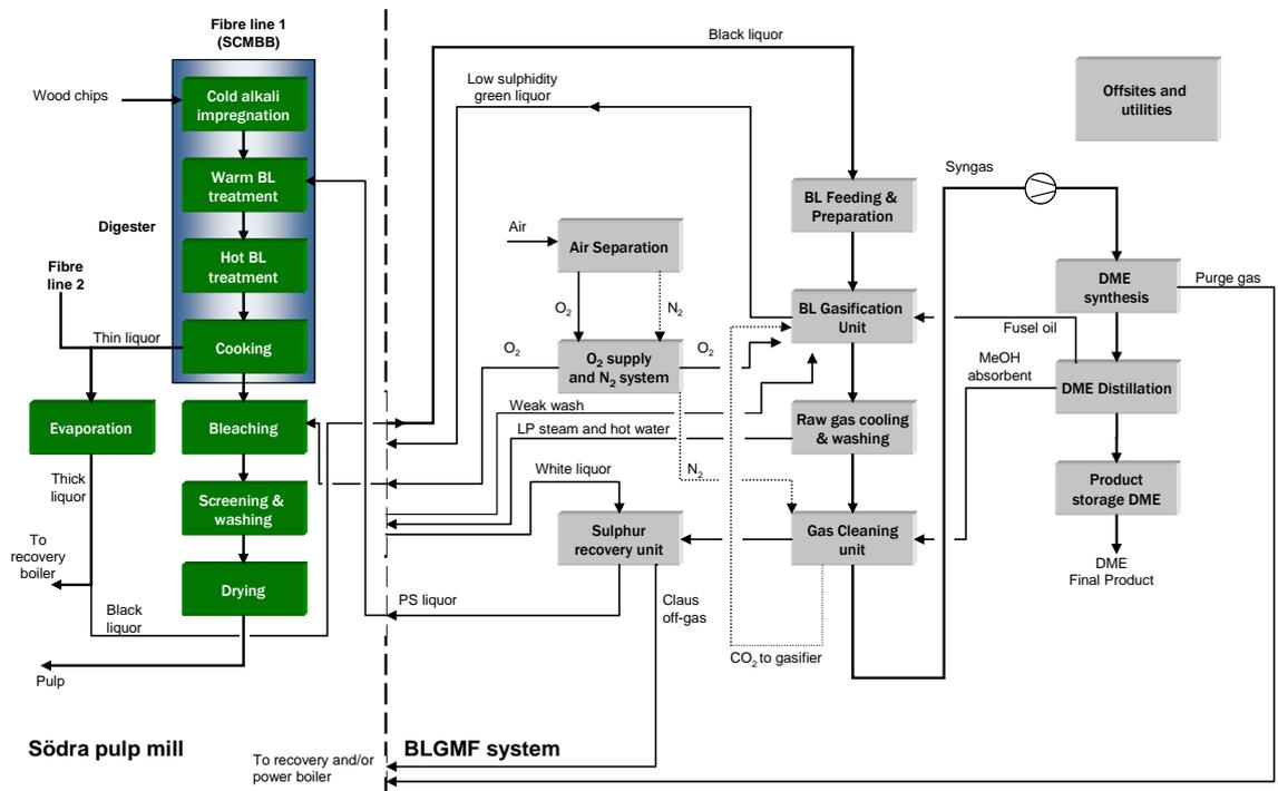
Figure 10 The BLGMF plant including the one-stage and simplified DME synthesis process
