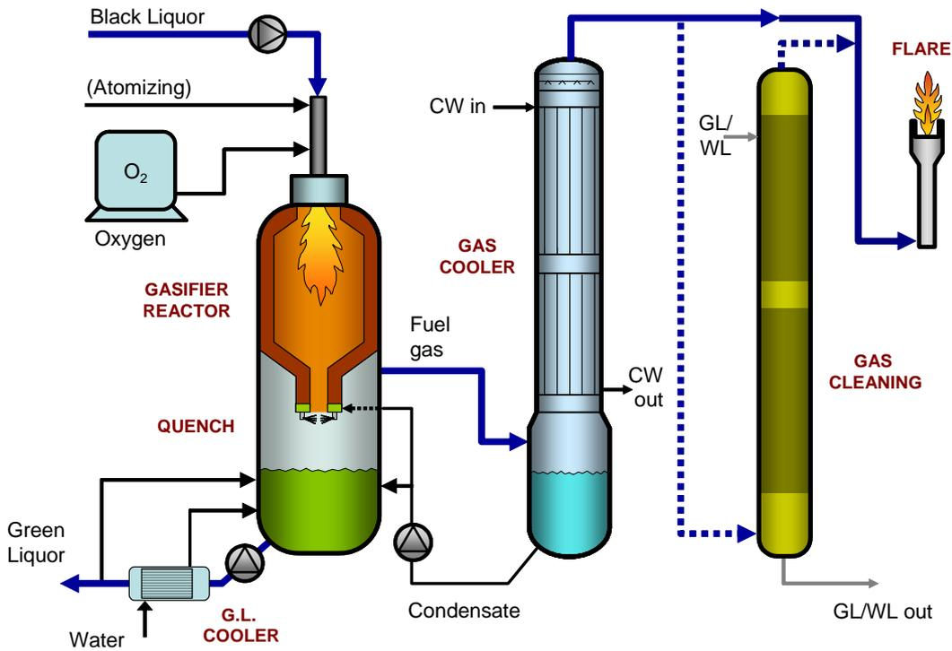
*Figure 3. The Chemrec Skoghall pilot plant for pressurized gasification of black liquor.*
