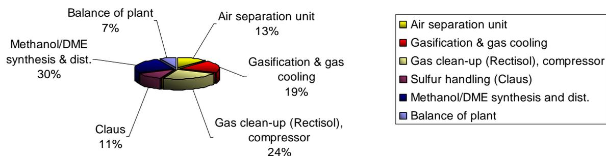
*Figure 6 Investment cost break-down on process units of the BLGMF plant.*
