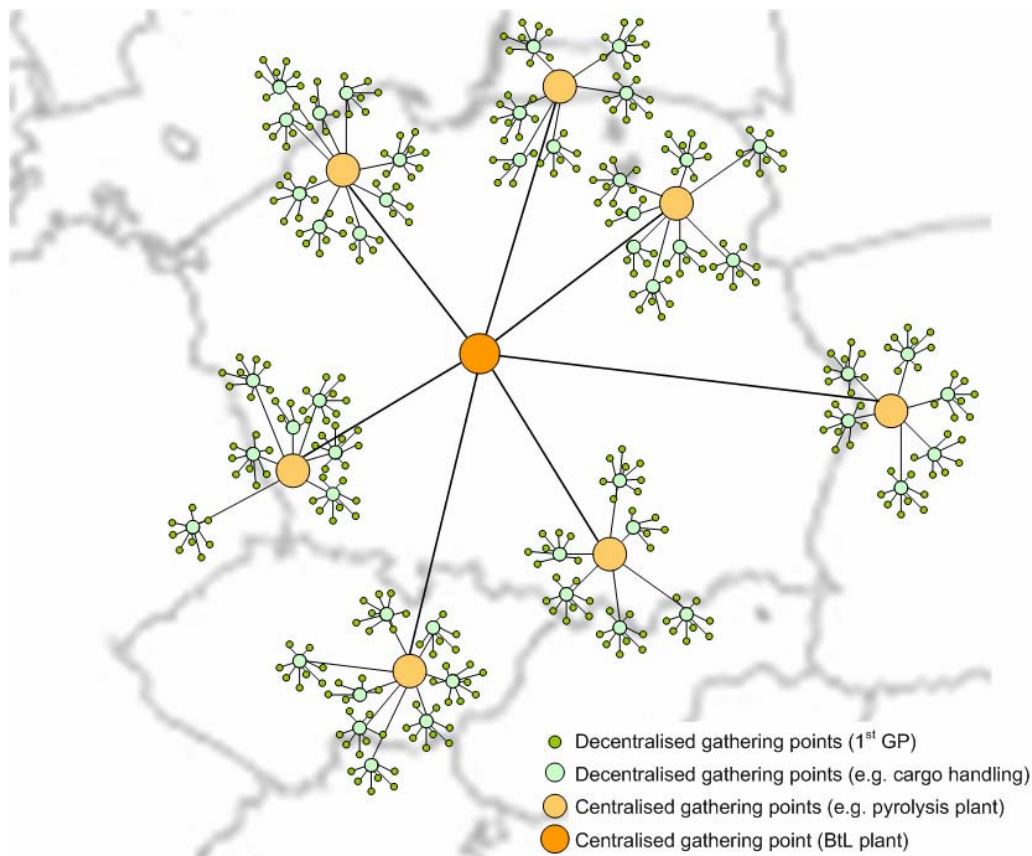
Figure 6-3 Principle of biomass provision level
